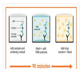
SimpleStep ELISA technology allows the formation of the antibodyantigen complex in one single step, reducing assay time to 90 minutes. Add samples or standards and antibody mix to wells all at once, incubate, wash, and add your final substrate. See protocol for a detailed step-by-step guide.
