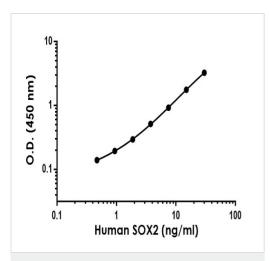
Example of human SOX2 standard curve in 1X Cell Extraction Buffer PTR.
