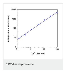
ZnCl<sub>2</sub> dose response was measured on a 96-well black plate with Zinc Quantification Kit (Fluorometric) (ab176725). As low as  $\sim$  0.2  $\mu$ M Zn<sup>2+</sup> can be detected with 5 minutes incubation time (n=3).
