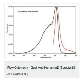
Fluorescence excitation and emission spectra of Allophycocyanin in 100mM sodium phosphate (pH7.2) + 1mM EDTA and 1mM sodium azide. The emission scan was taken with excitation at 630nm. The excitation scan was taken with an emission at 660nm. The curves were normailized to equalize peak heights.
