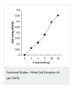
Whole cell extracts were prepared from MCF-7 cells using ab113475. Activity of SOD was measured using different amounts of the extract.
