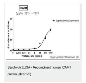
Standard curve for ICAM1 (Analyte: ab82125); dilution range 1pg/ml to 1µg/ml using Capture Antibody **ab2213** at 5µg/ml and Detector Antibody **ab7815** at 0.5µg/ml.
