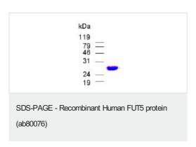
SDS PAGE analysis, 20% gel (Commassie blue staining) showing ab80076 at approximately 30kDa.
