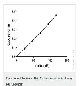
Standard curve (colorimetric): mean of duplicates (+/-SD) with background readings subtracted
