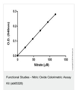
Standard curve (Colorimetric): mean of duplicates (+/-SD) with background readings subtracted
